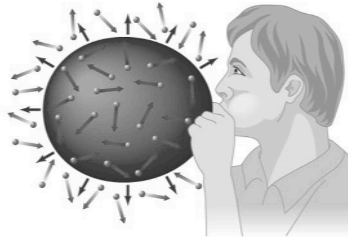
b Adding air molecules temporarily increases the pressure inside the balloon, so the balloon expands until pressure balance is restored.
